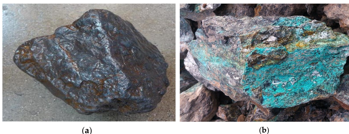
Figure 3. (a) Hematite iron ore sample from Afghanistan. (b) Copper oxide ore sample from Iran.
