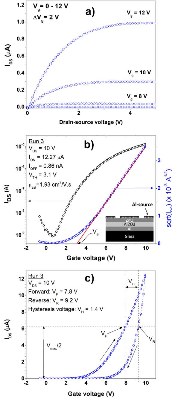
Figure 1: a) Output curves sweeping  $V_G$  from 0 to 12 V, in of 2 V steps; b) transfer curve and  $I_D^{1/2}$  vs.  $V_G$  for  $V_{DS} = +10 \text{ V}$ . Inset: schematic of the ZnO TFT structure; c) transfer curve, for  $V_{DS} = 10 \text{ V}$ , showing the hysteresis between forward and reverse scan; All curves were obtained from a ZnO TFT with anodised Al<sub>2</sub>O<sub>3</sub> prepared as specified in run # 3, Table 2
