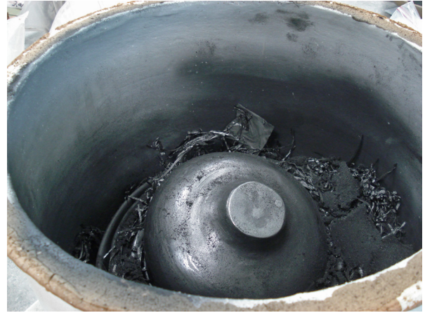
Figure 16: A way of creating reduced firing conditions: vessels are nested, filled and packed with burnable organic materials (© Laboratory for Material Culture Studies Leiden University).
