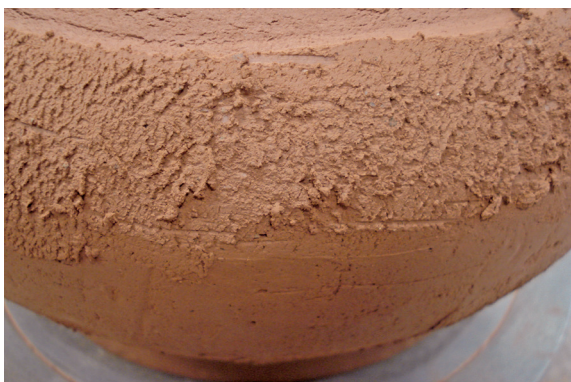
Figure 6: The surface is scraped to correct the shape and to remove excess clay (© Laboratory for Material Culture Studies Leiden University).
