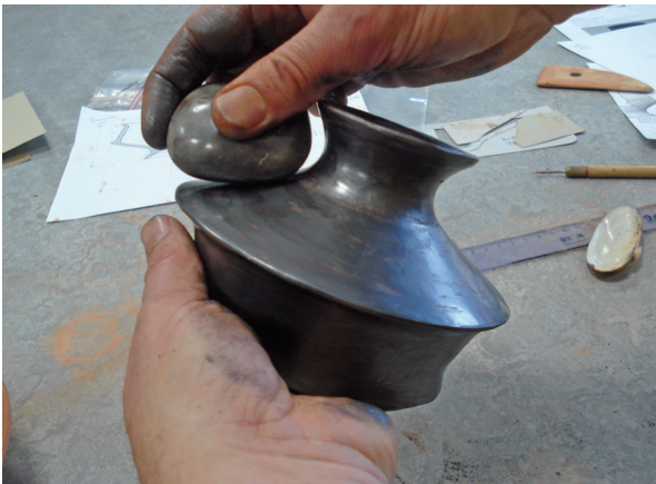
Figure 11: The leather-hard surface was polished with a polishing stone which consolidated the graphite. The pebble neatly fits in the curves in order to reach the entire surface (© V. Brigola).
