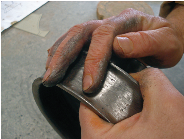
Figure 15: The application of graphite by rubbing the leather-hard surface with the powdered material (© V. Brigola).
