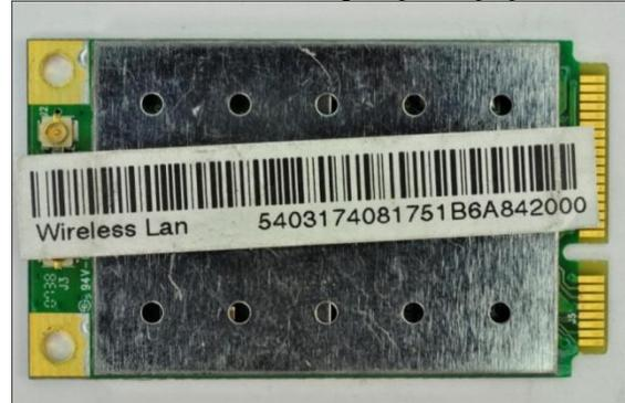
Gambar 3. Mini PCIe WLAN adapter
