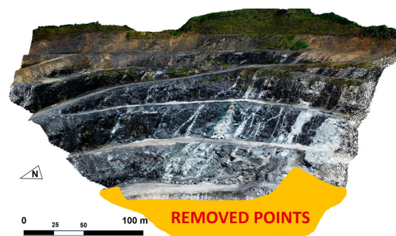
Figure 11. Open pit point cloud with the cut in orange. The new dense point cloud has 592,460 points and the new sparse cloud has 100,595 points. The cut region mainly consists of blasted rock.
