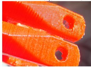
Figure 2.2: Difference between 0.3mm (top) and 0.15mm (bottom) layer thickness
