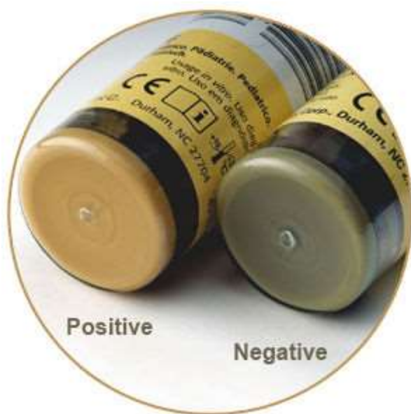
Figure 3. Liquid Emulsion Sensors (LES) at the bottom of each culture bottle visibly change color when the pH changes due to the rise in CO 2 as it is produced by microorganisms in BACT/ALERT® instruments.
