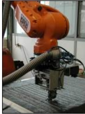
Figure 2-12 - Robot assisted stitching machine for CMC preforming available at Airbus Group Innovations.
