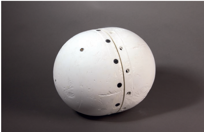
Figure 2-27 – Flight recorder protector made with WHIPOX ™ (WPX Faserkeramik GmbH, 2016).
