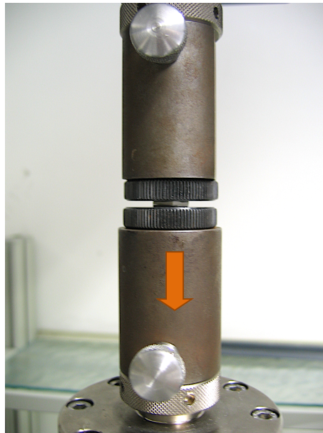
Figure 3-5 - Tensile test from an oxide ceramic matrix composite sample manufactured with Nextel™ 610 fiber, 3000 denier and sol gel suspension via filament winding and freeze gelation.
