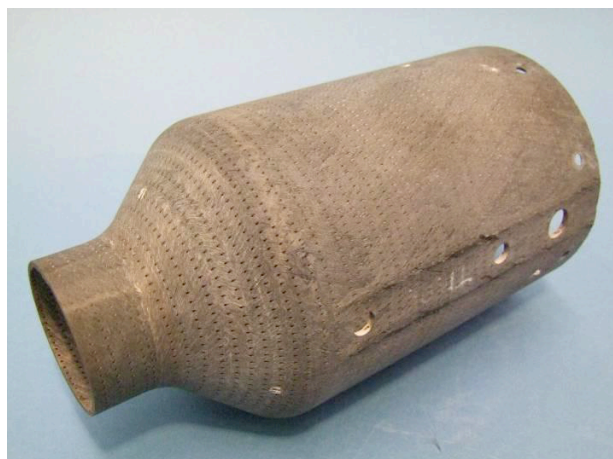
Figure 2-25 – Combustion chamber manufactured with UMOX™ after high temperature test.
