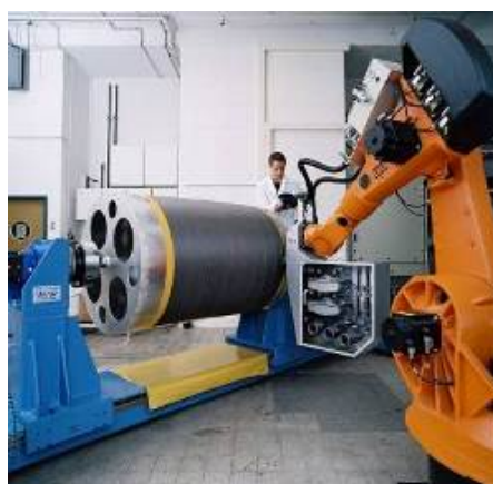
Figure 2-11 - Robot assisted 6+2-axis filament winding machine at Airbus Group Innovations.
