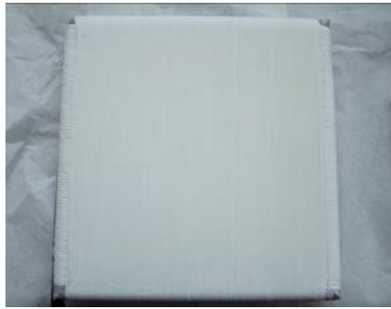
Figure 3-2 - Nextel™ 610 fibers with sol gel based suspension composite after filament winding and freeze gelation.
