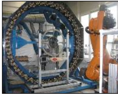
Figure 2-9 – Robot-assisted circular braiding machine at Airbus Group Innovations, Germany.
