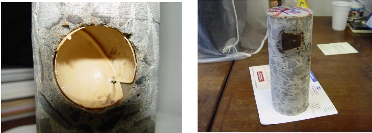
Fig.11 Core samples showing the table tennis ball and the small piece of wood
