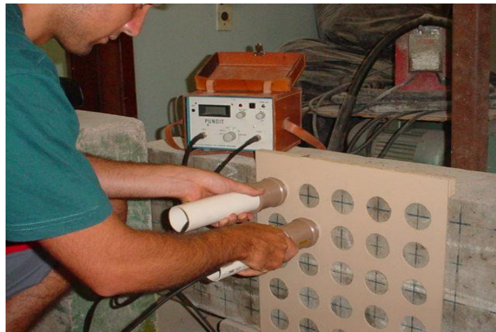
Figure 5. View of the execution of the UPV test.
