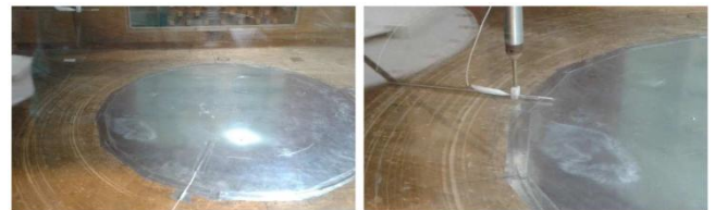
Figure 4. Experimental section II and positioning of the hot wire anemometer
