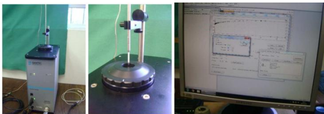
Figure 2. Calibration system and process of an anemometer probe
