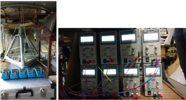
Figure 6. Temperature control of the upper sheet (left) and power supply of the Peltier elements with constant DC current (right)
