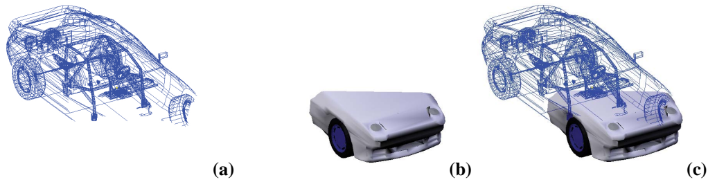
Figure 10: As the slicing technique is used, parts of the model between the near and far clipping planes are moved from the back layer (a) to the front layer (b) to provide the combined MLD view (c).
