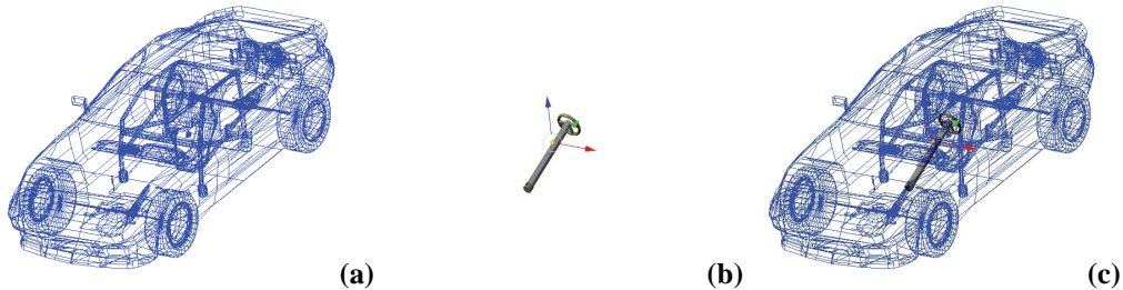
Figure 2: Using the object isolation technique, the object of interest can be edited on the front layer (b) while context of the rest of the model is shown on the back layer (a).
