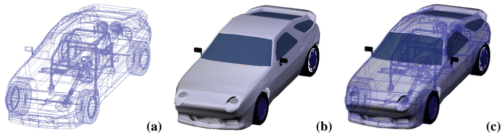
Figure 1: The initial view of the 3D model of a car on MLD, showing the back layer (a), front layer (b) and combined view (c).
