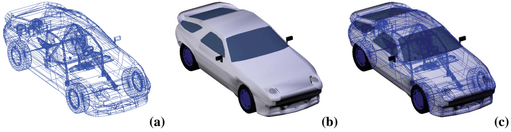
Figure 8: View of the model on MLD before the slicing technique is applied, back layer (a), front layer (b) and the combined view (c).
