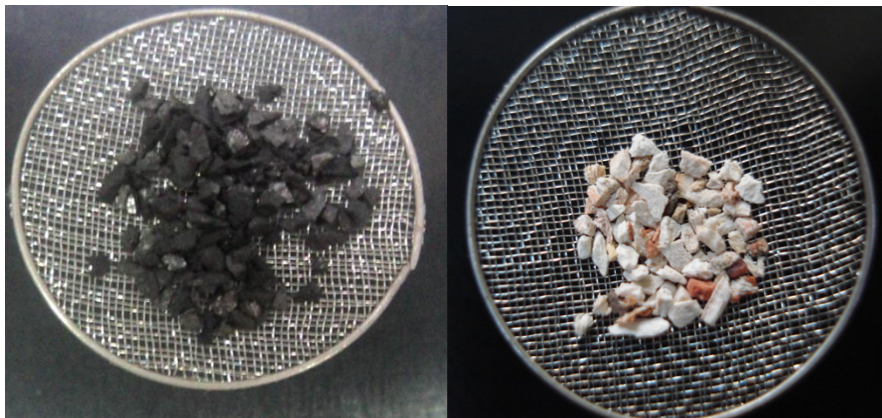
Figure 10: Char before oxy-fuel combustion and ash after oxy-fuel combustion.
