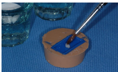
Figure 2. Filling the matrix with acrylic resin through the brush technique.
