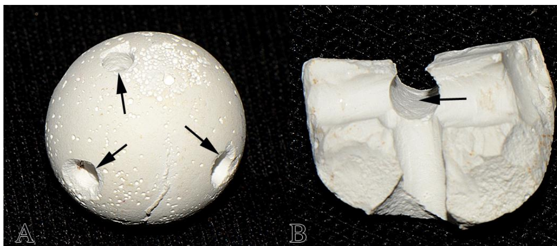
Figure 1. Surface of the double-setting alpha-tricalcium phosphate bone cement of interconnecting channels implant. A. External. B. Internal.
