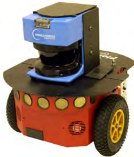
Figure 4.1: Robot used in the experiments: a Pioneer 3-DX equipped with a SICK LMS-200 laser rangefinder.
