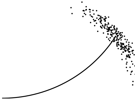
Figure 2.4: Example of sampling based on the probabilistic motion model. Figure extracted from (MONTEMERLO; THRUN, 2007).
