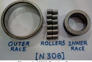
Figura 1: N308 Bearing Parts
