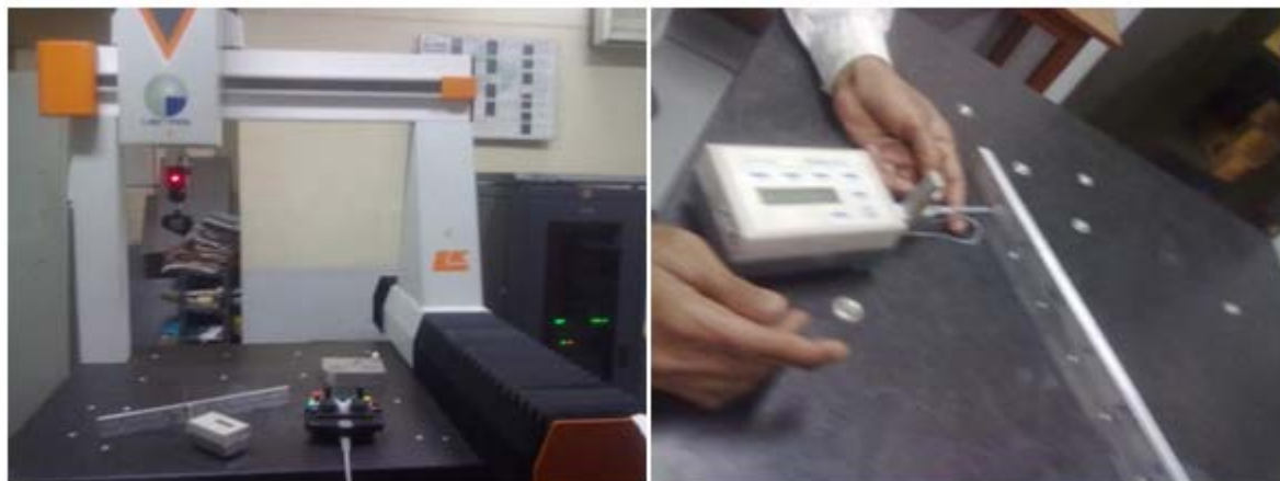
Figure3: Coordinate Measuring Machine and surface analyser of Talysurf 50
