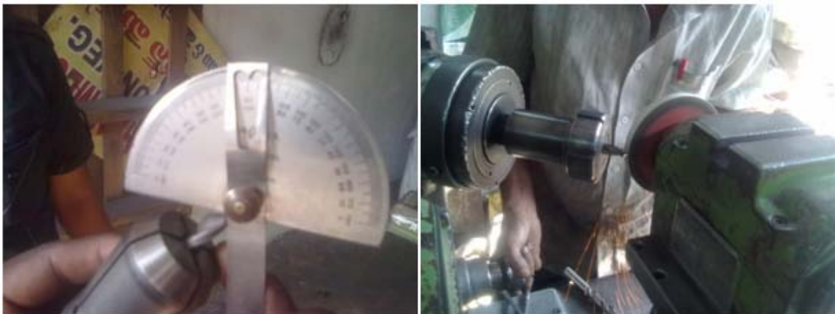
Figure 2: Alteration of drill tool geometry using Tool and Cutter grinder
