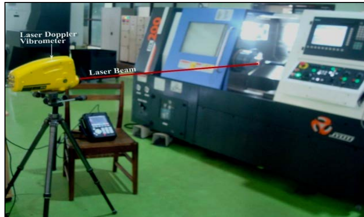
Figure 6 :Measurement of rotating work piece vibration using LDV Source: Venkatarao, Murthy and Mohanrao (2014)
