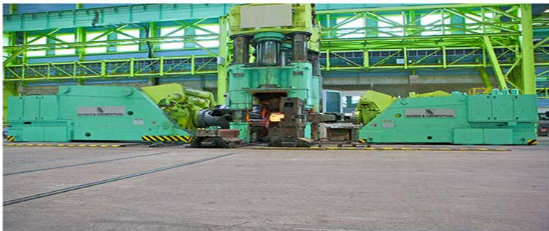
Figure 2: Forging Manipulator (Rail Mobile) Source: Dango & Dienenthal
