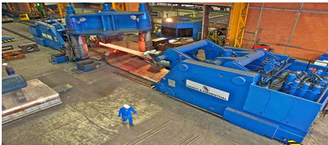
Figure 3: Forging Manipulator (Rail Mobile) Source: Dango & Dienenthal
