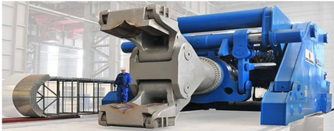
Figure 1: Forging Manipulator (Rail Mobile) Source: Dango & Dienenthal
