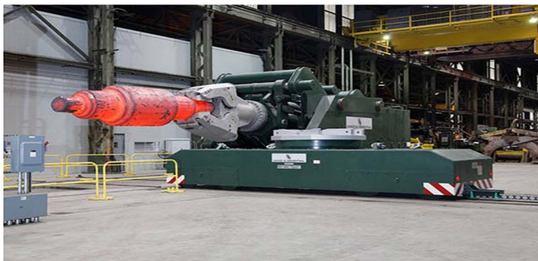
Figure 12: Forging Manipulator (Rail Mobile) Source: Dango & Dienenthal
