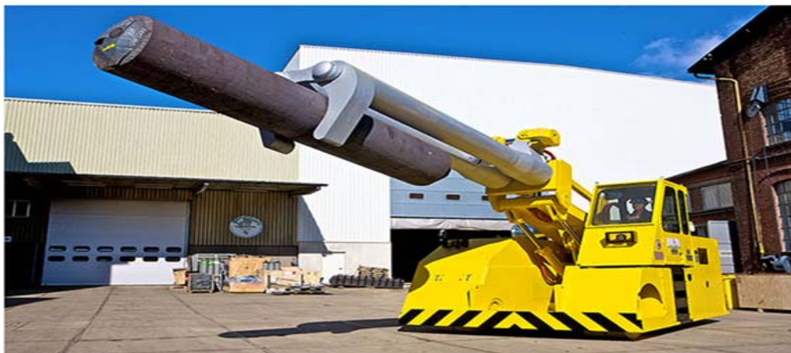
Figure 11: Forging Manipulator (Independent Mobile) Source: Dango & Dienenthal
