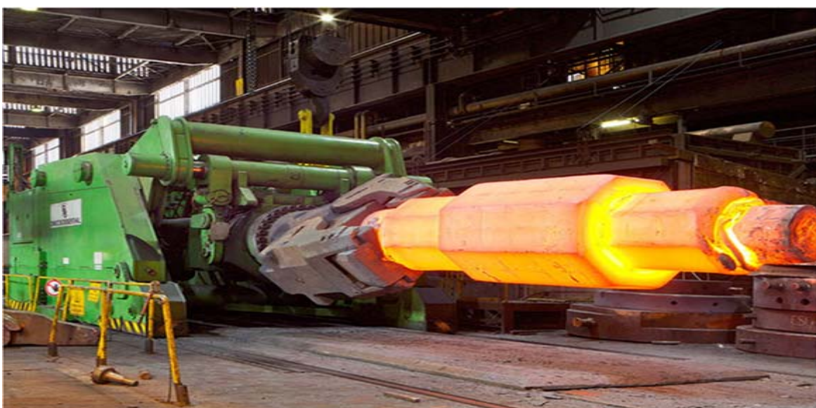
Figure 6: Forging Manipulator (Rail Mobile) Source: Dango & Dienenthal
