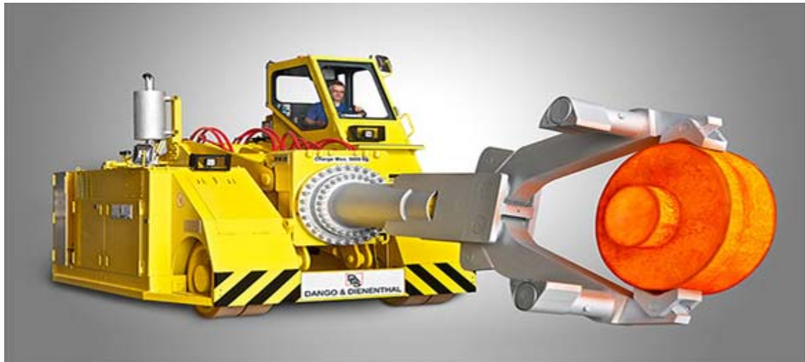
Figure 10: Forging Manipulator (Independent Mobile) Source: Dango & Dienenthal
