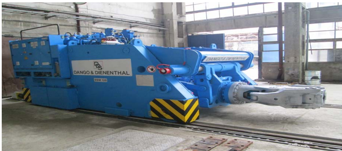
Figure 13: Forging Manipulator (Rail Mobile)
