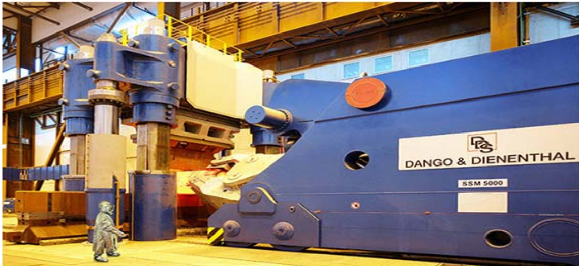
Figure 4: Forging Manipulator (Rail Mobile) Source: Dango & Dienenthal
