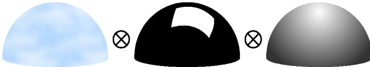
Figure 2: To determine the illumination of a point over a surface, it is necessary to integrate, along with its material properties, the lighting function (leftmost), the visibility function (center) and the geometric factor (rightmost).
