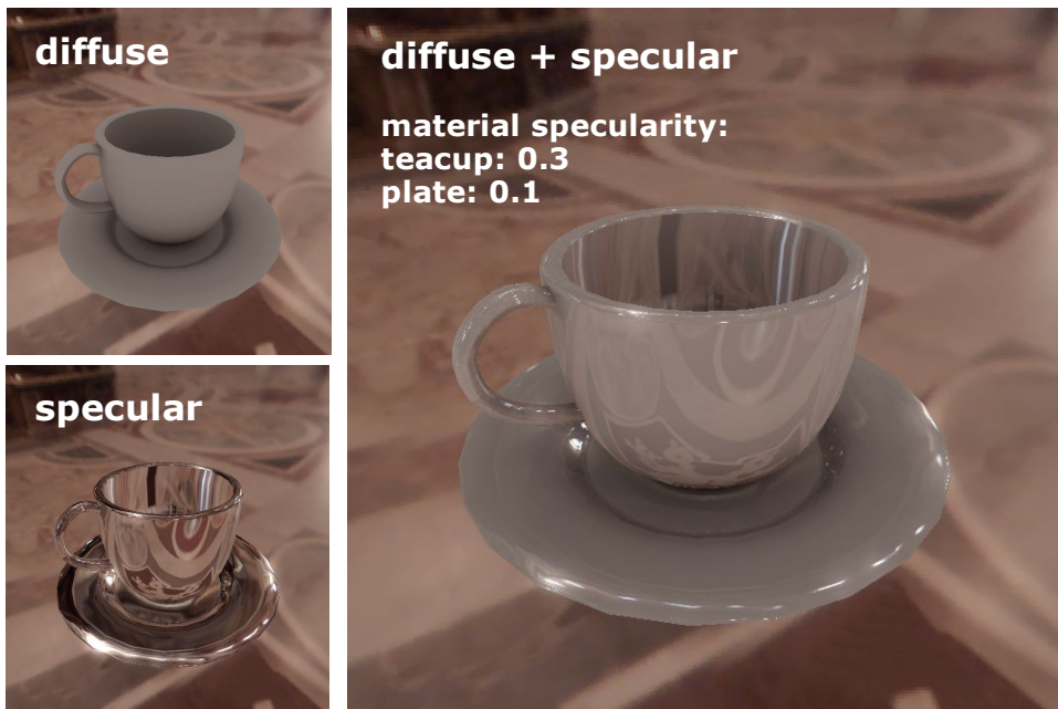
Figure 11: A teacup rendered using both diffuse PRT and reflection mapping. An high dynamic range image was used for lighting function and environment texture, so tone mapping was employed to properly exhibits the generated image.
