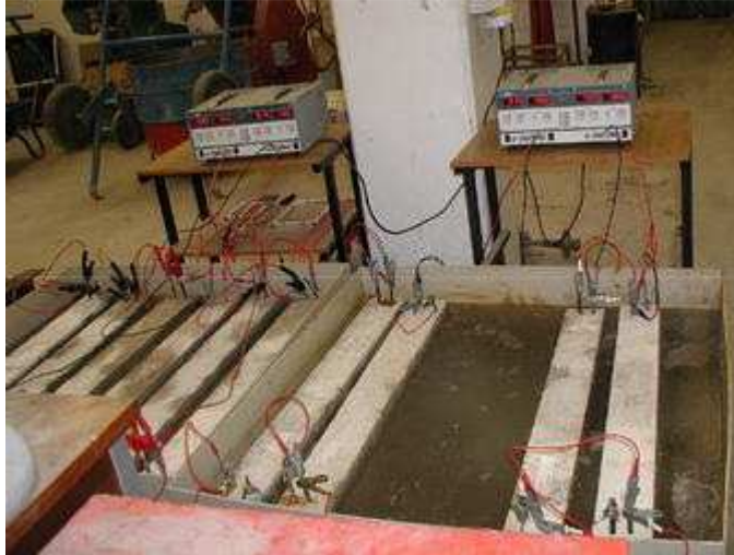
Fig. 2: Reinforced concrete beams undergoing main reinforcement corrosion
