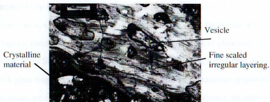
Figure 2.4. Photomicrograph of Ötting quarry impact melt glass. Showing streaky layered structure, inclusions of crystalline material and vesicles. Magnification x5. (Field of view 20 mm).
