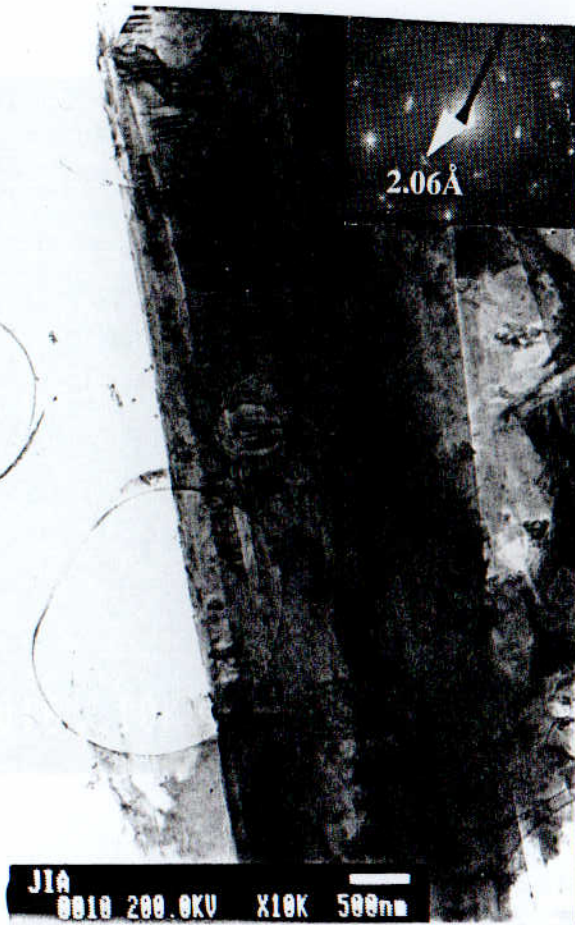
Figure 3.7. Bright field transmission electron microscope (BFTEM) image of an elongate, layered diamond from the Aumühle quarry gneiss. [x10 k, 200 kV, scalebar 500 nm].
