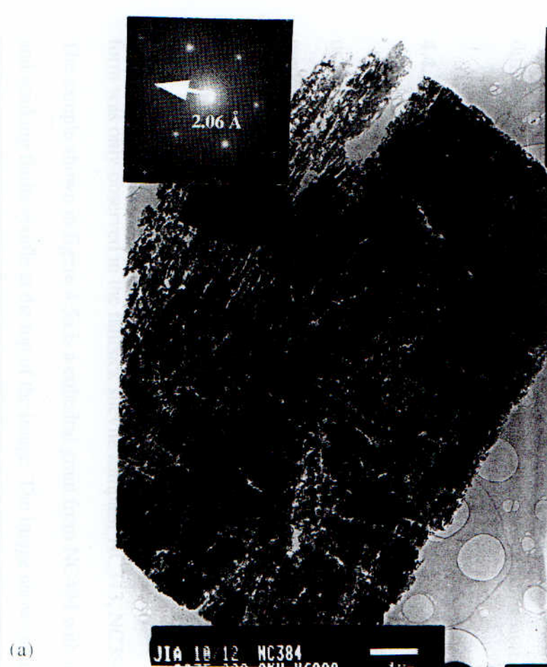
Figure 4.5. (a) BFTEM image of a blocky fractured diamond from NC494 showing skeletal etched structure at the top of the grain and faint stacking fault features below the opaque area. Inset SAED shows diamond 2.06 Å. [x 6 k, 200 kV, scalebar 1 μm]. (b) BFTEM image of skeletal etched diamond grain from NC384. Inset SAED shows diamond 2.06 Å. [x 8 k, 200 kV, scalebar 1 μm].
