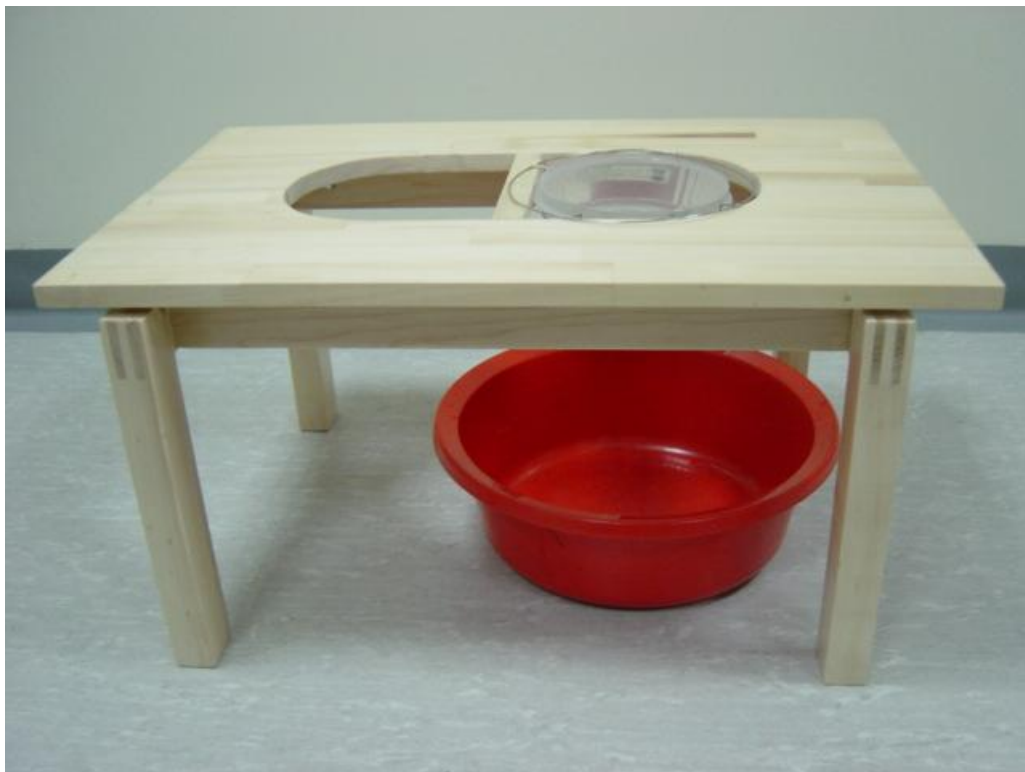
Figure 2.11 Water displacement system for live models
