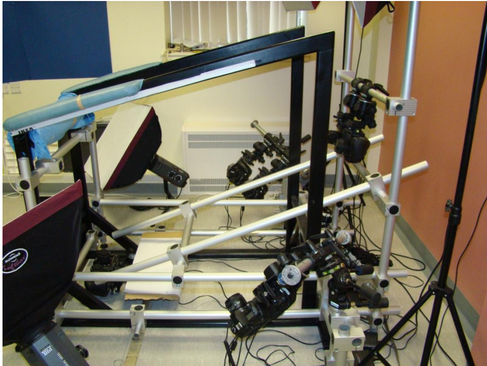
Figure 2.13 Eight high resolution digital cameras used in camera system
