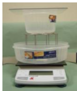
Fig. 6. Water displacement system for plaster breast model measurement
