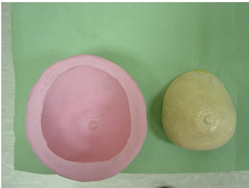
Figure 2.3 Rubber bowls for the molding of plaster models
