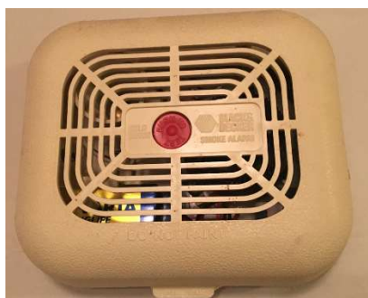
Figure 8. Smoke detector Photo: VTT
