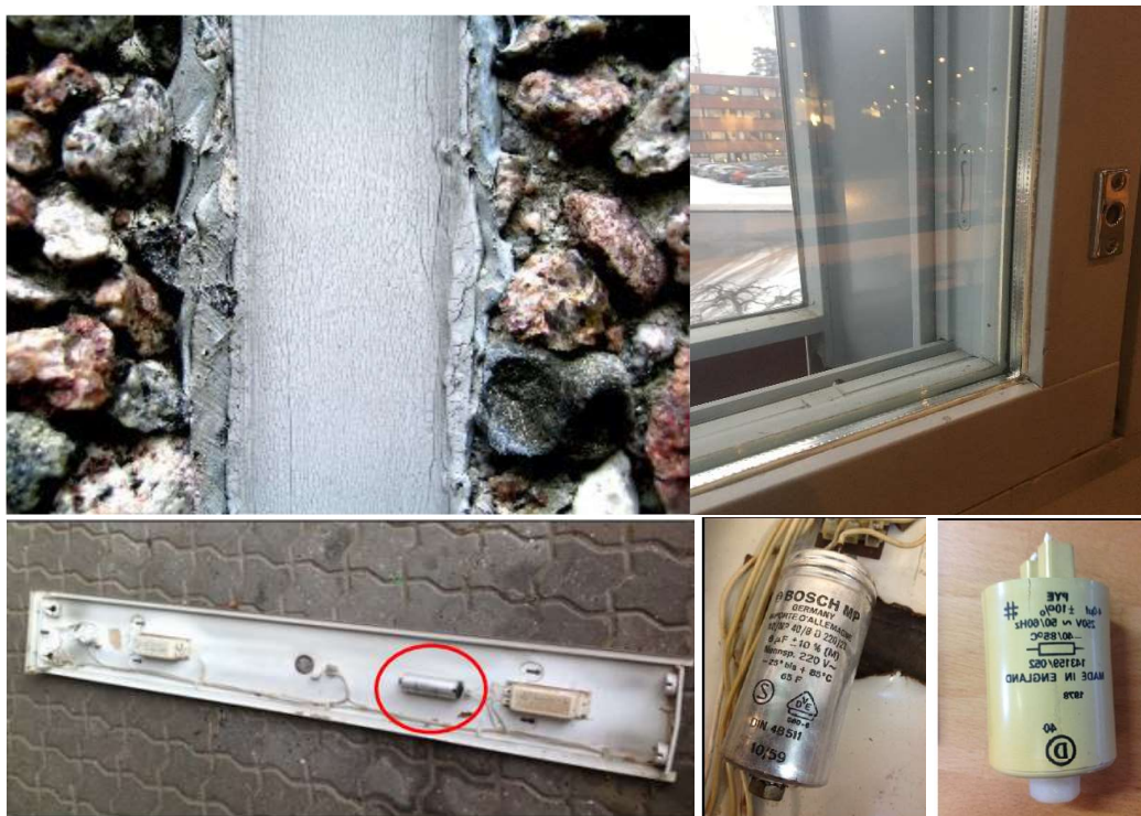
Figure 4. PCB containing sealants. PCB containing condensers in lamps (marked with red circle) and examples of condensers with manufacturing year visible. Photos: Jarno Komulainen, Vahanen Building Physics Ltd (upper left), VTT OY (upper left) & Danish EPA report Miljostyrelsen nr 10, 201518 (photos below)
