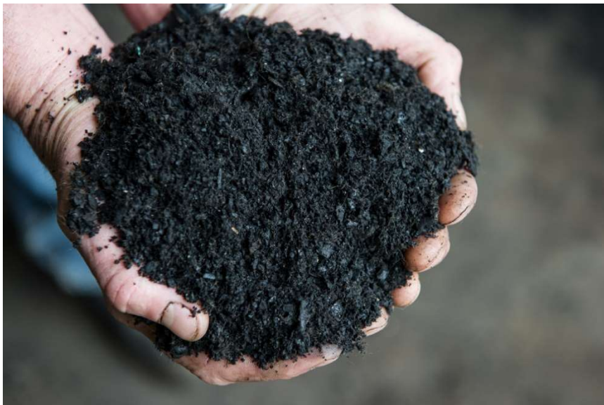
Figure 26. Recycled bituminous roofing waste for use in asphalt, produced by BituRec.
