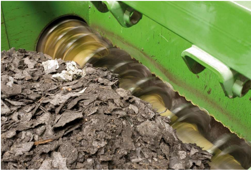
Figure 25. Shredding of bituminous roofing demolition waste in the BiELSO plant.
