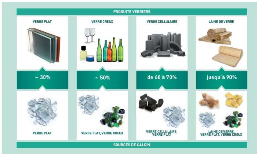
Figure 15. Glass fractions and their recycling route 30 .
