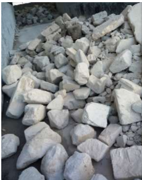
Figure 27. Sorted AAC from demolition works that is suitable for recycling in new AAC 80 .
