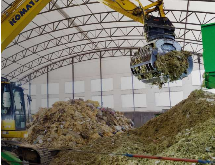
Figure 24. Stone wool waste for recycling 66 .
