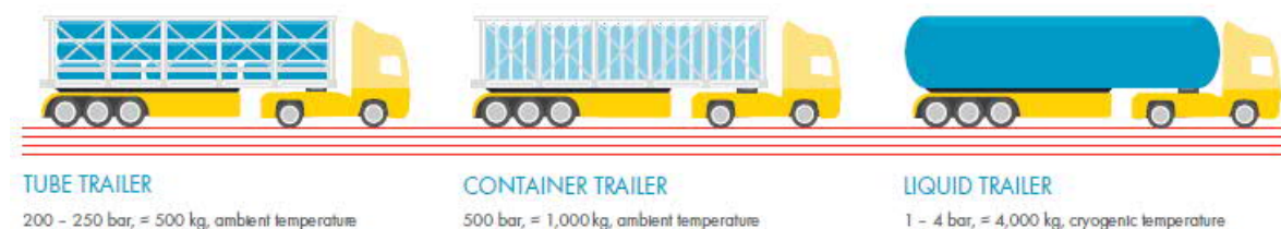
Figure 4. Existing road transport options for distributing hydrogen. (Shell 2017)
