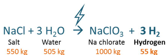
Figure 22. Overall reaction for an ideal chlorate plant.
