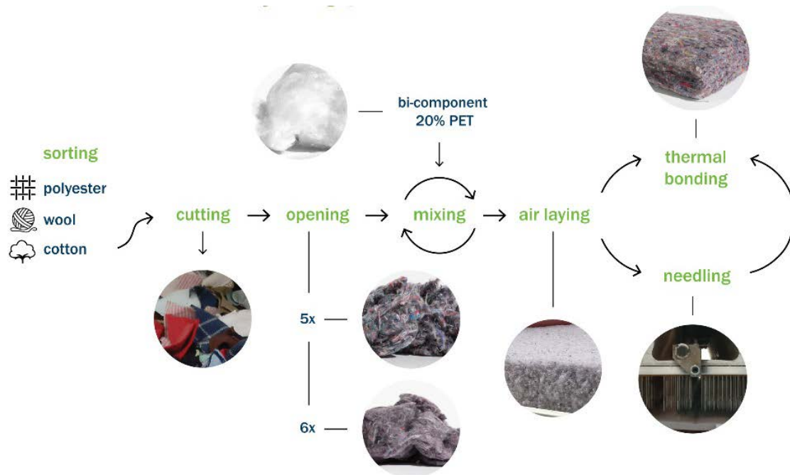
Figure 33 Demonstration of the mechanical recycling process at Laroche’s technical centre. Process description by Pirita Hyrkkäinen, Lahti University of Applied Sciences
