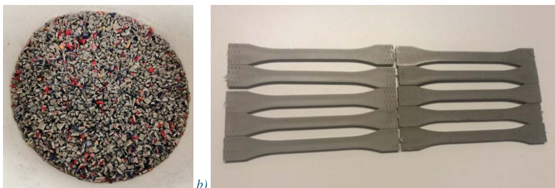
Figure 49 a) Prepared granulate-mix for extrusion, and b) Injection moulded test samples for mechanical testing: recycled PP on left and 90 % recycled PP + 10 % textile fibres on right
