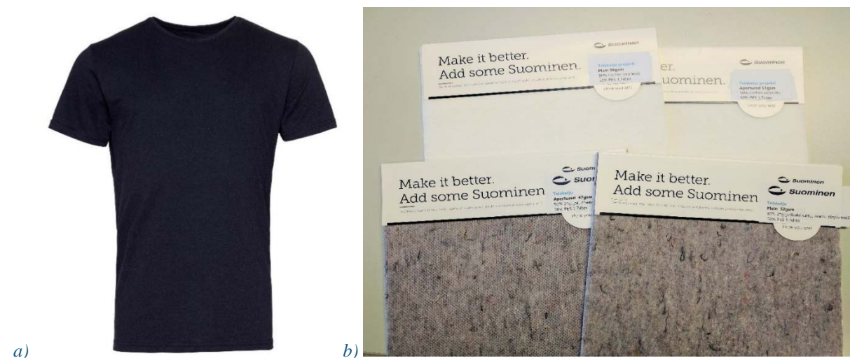
Figure 36 a) T-shirt made of yarn that consisted recycled post-consumer textile waste (20 %), pre-consumer textile waste (40 %) and recycled polyester (40 %); b) Nonwoven prototypes made of recycled and bleached IFC fibres and polyester (upper samples) and recycled fibres from Laroche demo and polyester (lower samples)
