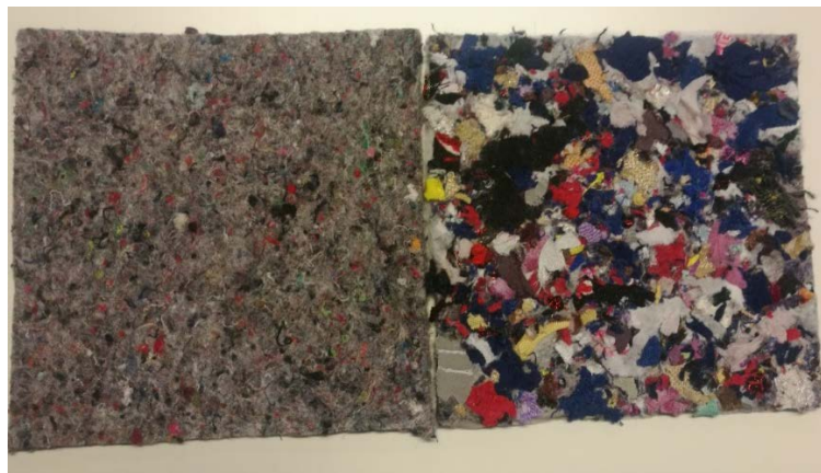
Figure 46 Materials produced with ArtImmersion demo: Compressed polyester sheet from materials obtained from Laroche trials on left and sheets covered with crushed textile pieces on right
