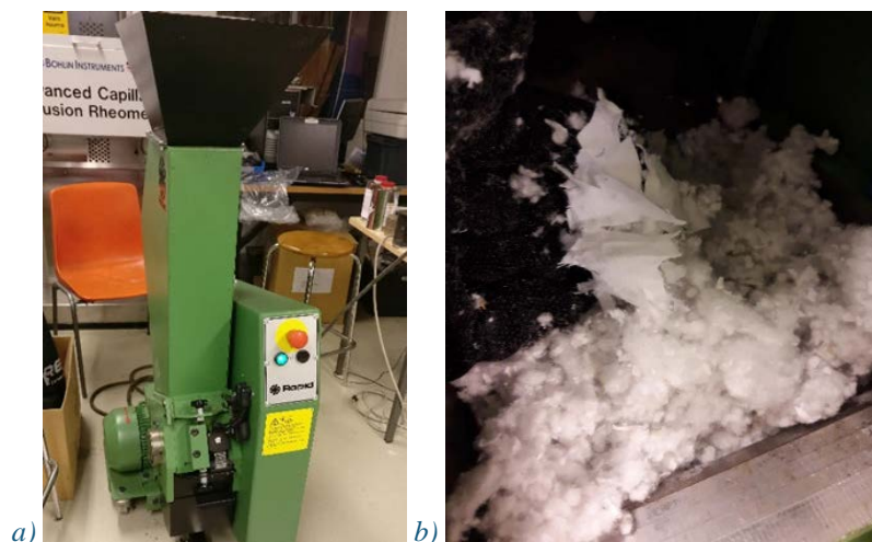
Figure 51 a) A crusher used in the trial was not effective enough to produce homogenous material. B) Large fabric pieces from the outer layers of pillows and duvets exist among polyester fibres after crushing
