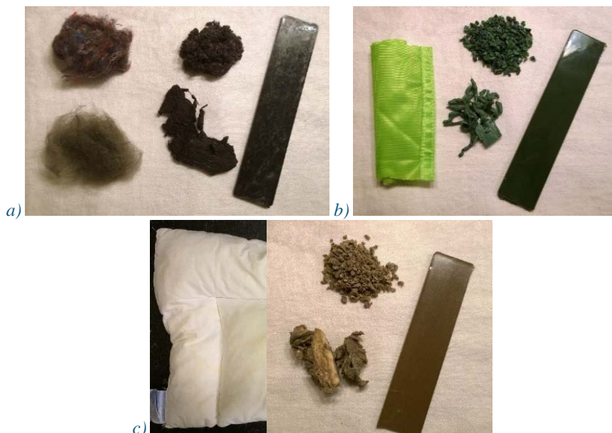
Figure 54 Processing steps from starting material to injection moulded bar a) 60 % polyester post-consumer + 40 % PP industrial waste b) 100 % polyester stripes c) pillow (filling 100 % polyester and outer surface 100 % cotton)
