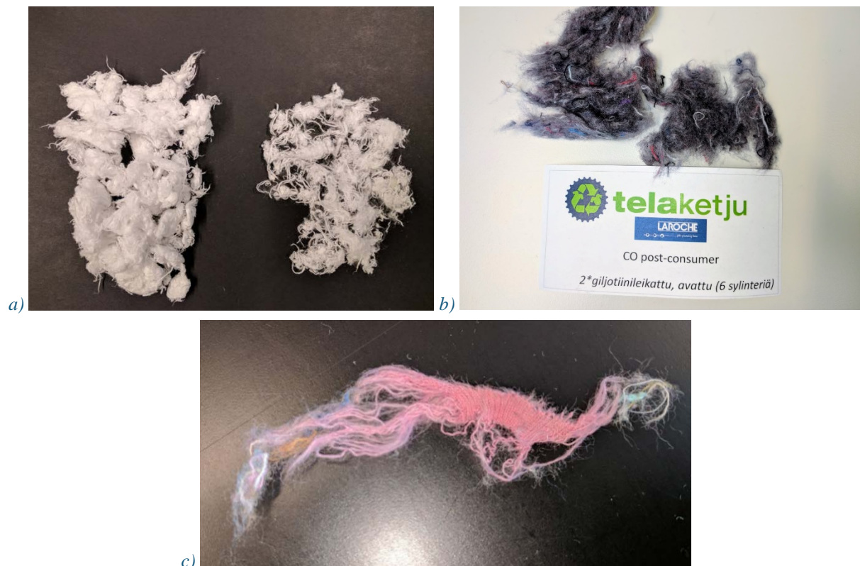
Figure 37 a) Mechanically recycled and bleached cotton fibres (left), and some fibres were lost in the carding process (right); b) Mechanically recycled cotton fibres from Laroche demo; c) Unopened material from the Laroche demo in the recycled fibre mix
