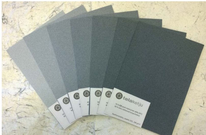
Figure 40 Samples produced from post-consumer CO-dust and pulp with foam laying technology. The CO fibre content ranged from 10 % (left) to 70 % (right)
