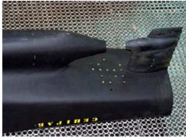
Fig. 3.1.1.3.- Dummy model for cavitation tests with CRP-POD system.
