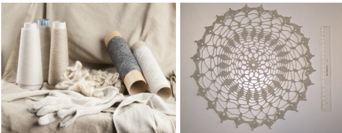
Figure 8 Recycled CCA fibres and demonstrated products from chemically recycled cotton regenerated into CCA fibres
