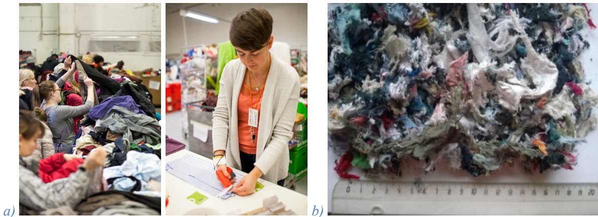
Figure 4 a) Sorting of post-consumer materials in HMARC, and b) grinded textile materials
