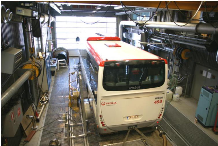
Fig. 1 View of the test facility, the CVS dilution tunnel can be seen in the upper right-hand corner
