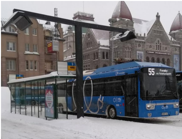
Fig 8 A Linkker bus at a charging station in Helsinki (January 2019)
