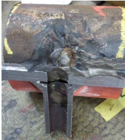
Figure 5. A section of a failed boiler tube.
