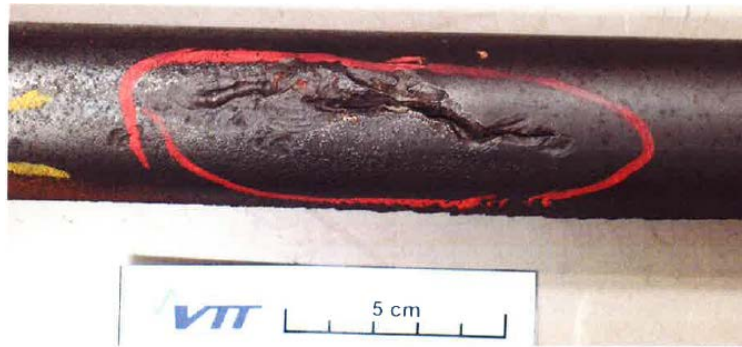
Figure 9. Failed superheater tube with indications of primary corrosion damage [11].
