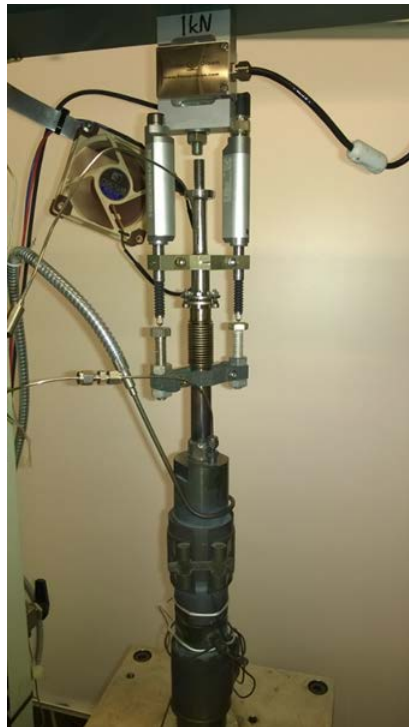
Figure 1. Small Punch creep rig at VTT with thermal insulation removed. Parts from above: load cell, displacement transducers, loading bar, metallic bellow and the rig with two heating cables clamped in place by stainless steel sheets.
