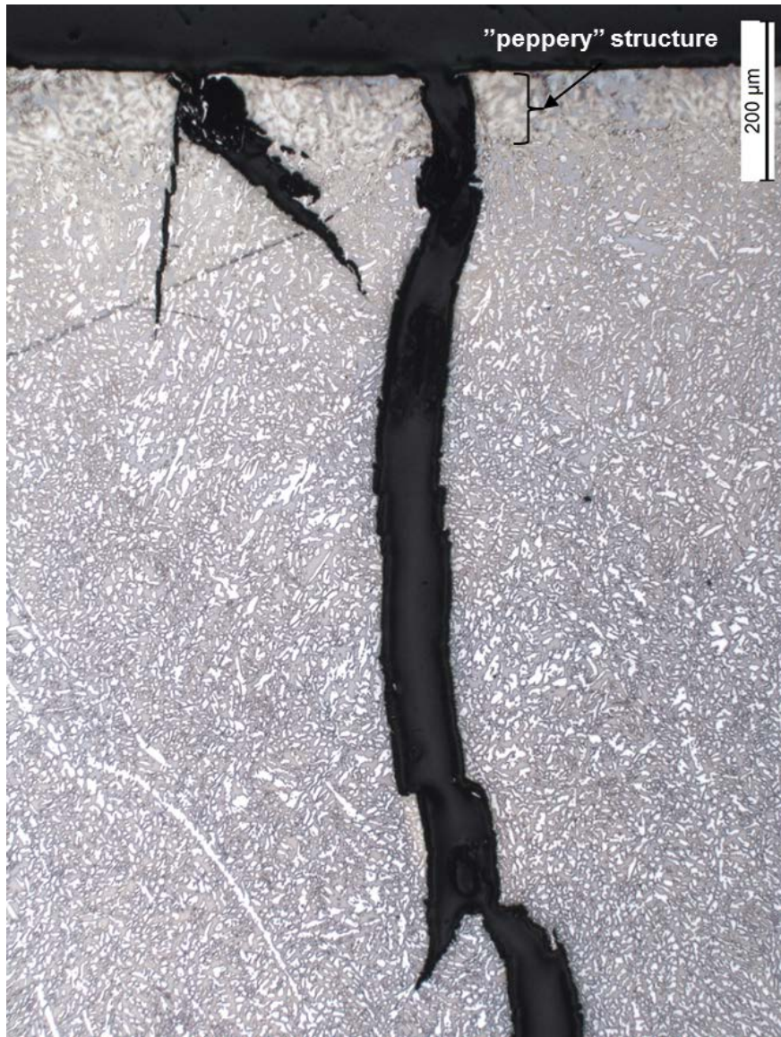
Figure 7. Crack initiation at the outer surface of the specimen close to the weldment, thin layer with “peppery” structure, several individual microcracks at the surface, crack branching along the propagation path.
