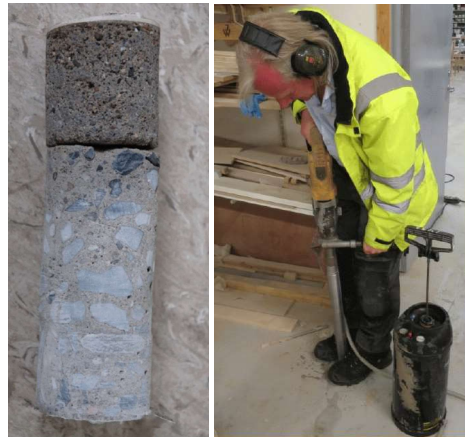
Figure. Sampling by drilling (photos: Eirik Waerner, Multiconsult, Norway)
