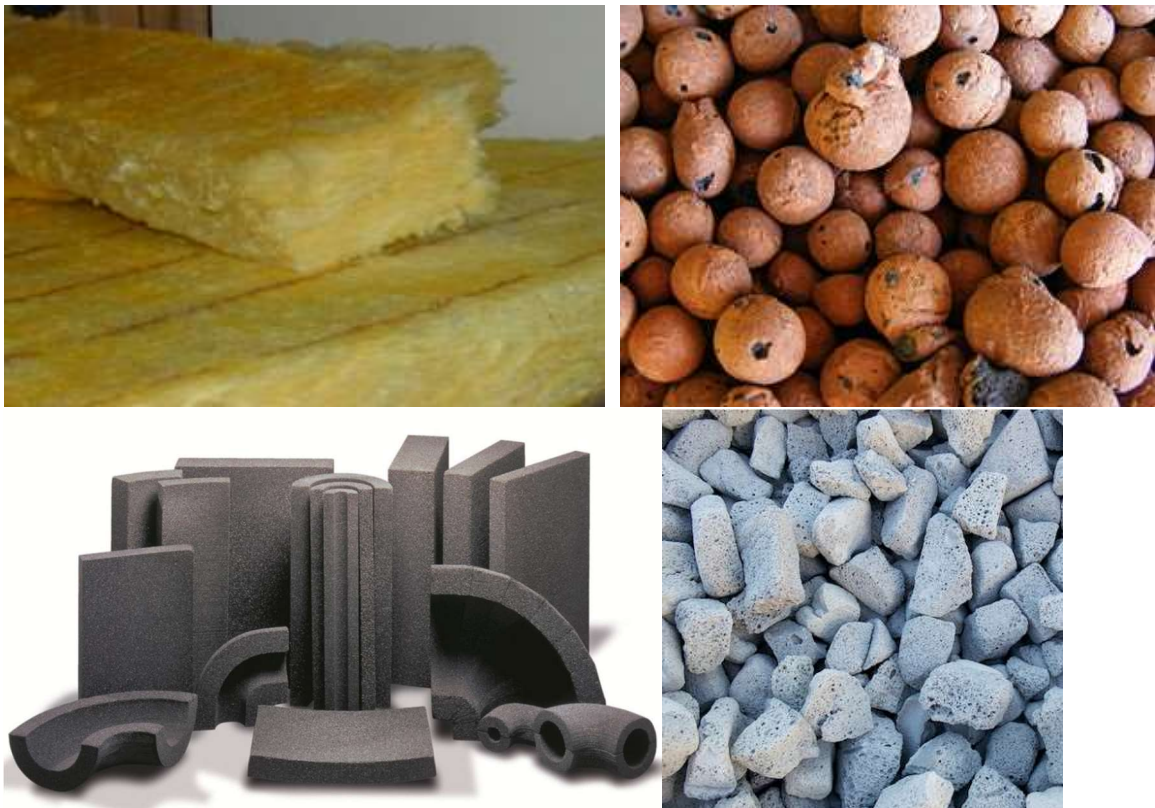
Figure 23. Mineral insulation products (top left: glass wool, top right: expanded clay aggregates, bottom: foam glass).
