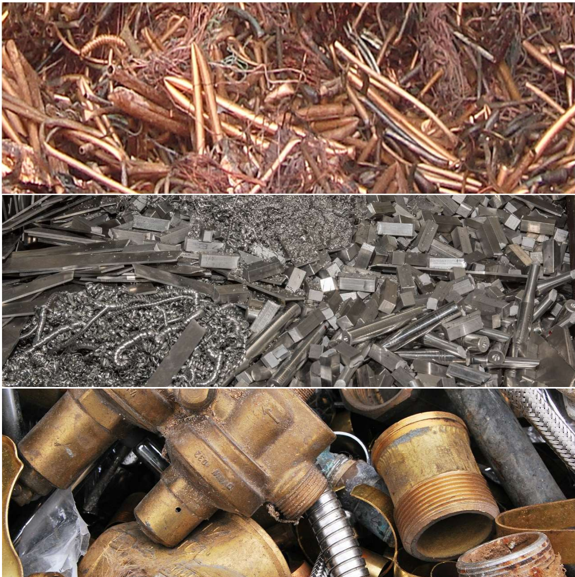
Figure 10. Typical copper (top), aluminium (middle) and brass (bottom) scrap.
