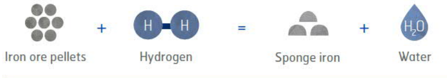
Figure 14. Hydrogen based direct reduction of iron ore. (HYBRIT 2018)
