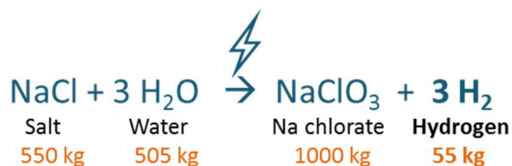
Figure 22. Overall reaction for an ideal chlorate plant.
