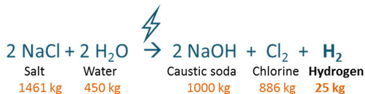
Figure 21. Overall reaction for an ideal chlor-alkali plant.
