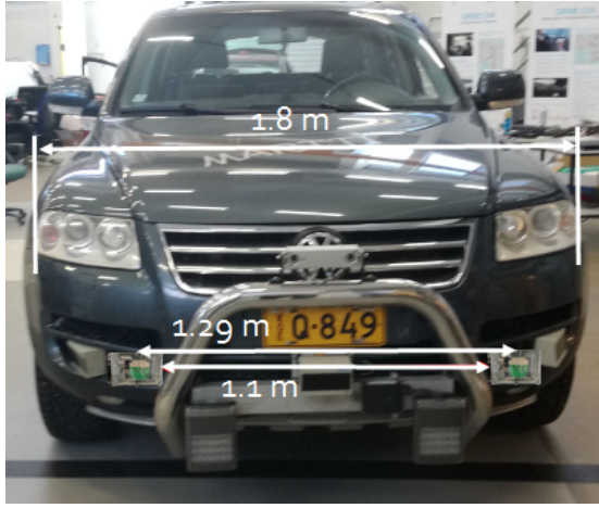
Fig. 2: The maximum distance of the radars in the Martti robot car.
