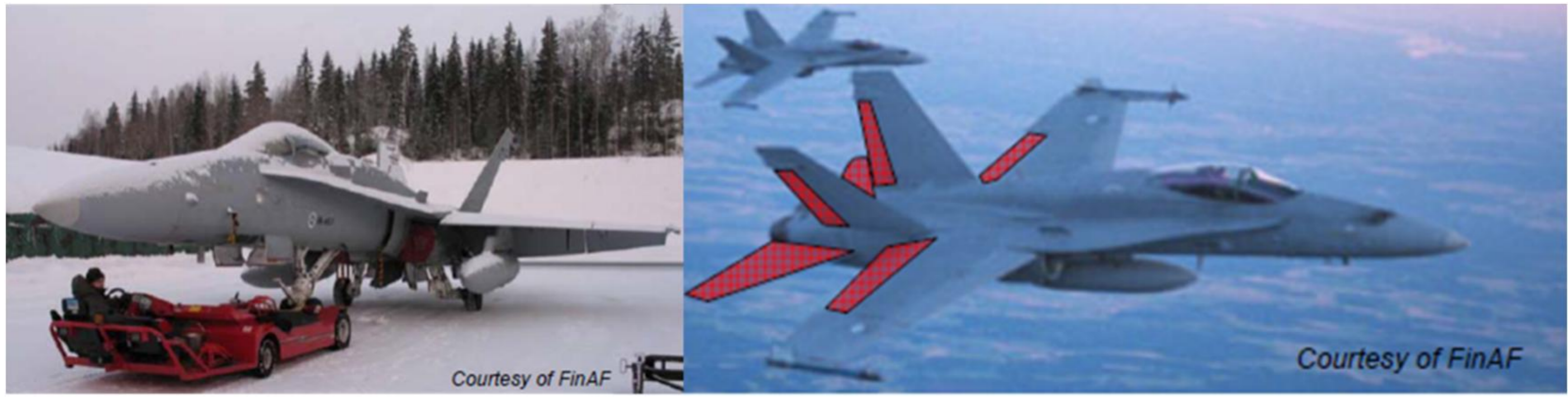
Figure 20: The optimal thermographic inspection exploiting phase transition of water. Left: To succeed in the thermographic inspections, it is of paramount importance to ensure adequate cooling (freezing) of the aircraft before starting of the measurements. Right: The inspection consisted of six different flight surfaces (10 locations) in one sequence of inspection checks. Picture by courtesy of the FINAF.
