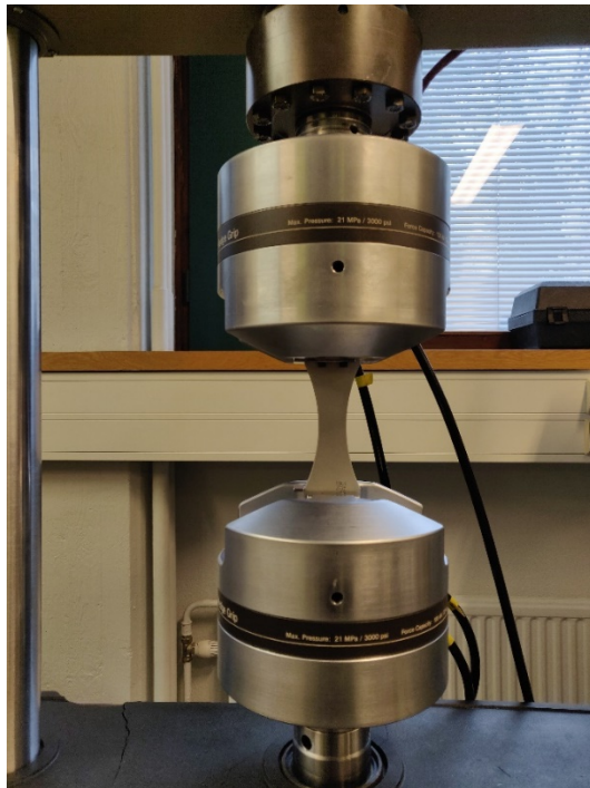
Figure 36: A dog-bone specimen in the variable amplitude fatigue test. Figure courtesy of Aalto University.
