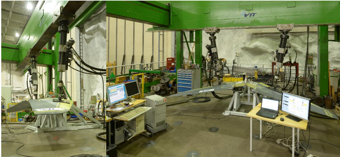
Figure 34: The test set-up of the FINAF Hawk tailplane. Figure courtesy of Eurofins Expert Services.
