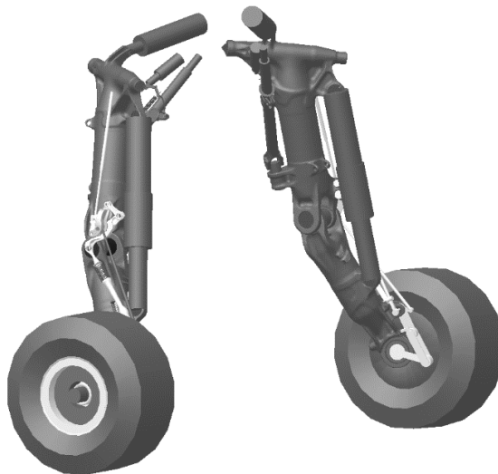
Figure 66: Updated Main Landing Gear model of the FINAF's F/A-18C/D Hornet. Figure courtesy of Patria Aviation.
