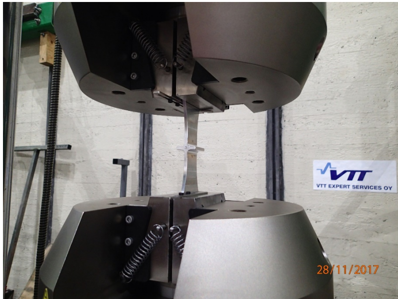
Figure 31: POD test specimen under cycling in the universal test machine. Figure courtesy of VTT.
