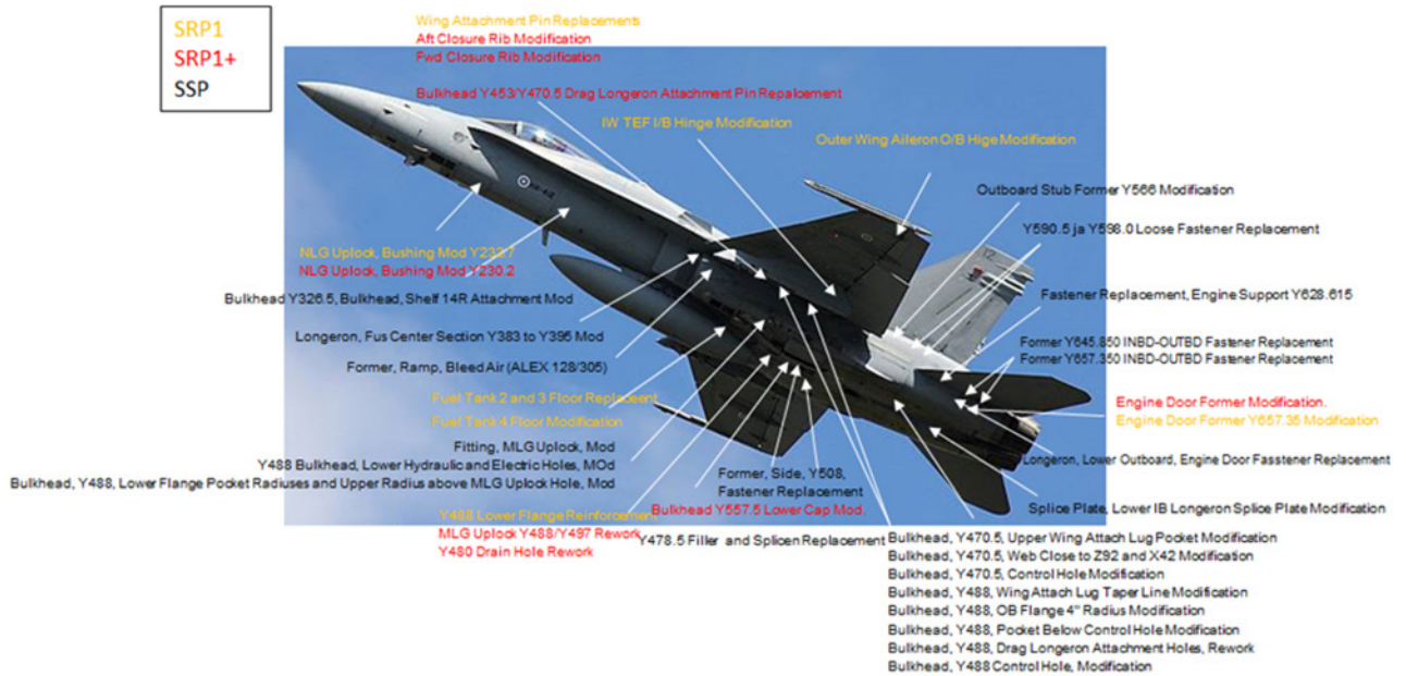
Figure 28: The overview of the SRP1, SRP1+ and SSP modification locations. Figure courtesy of Patria Aviation.
