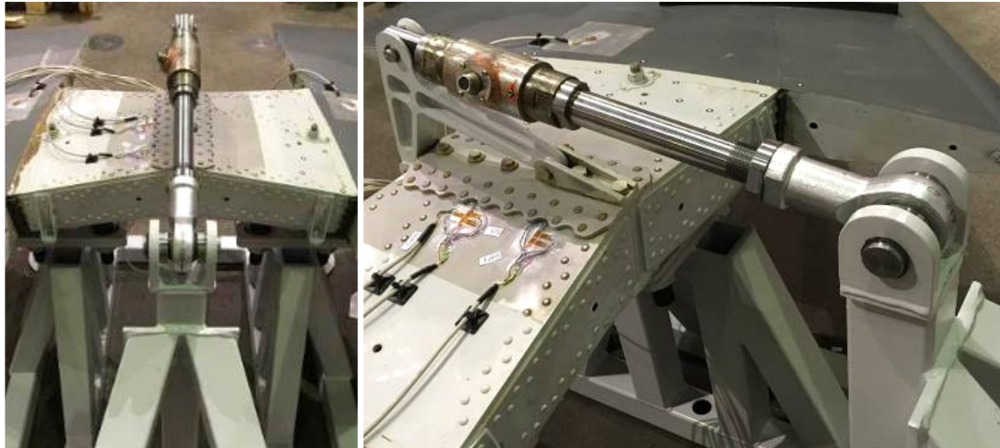
Figure 35: The critical detail of the FINAF Hawk tailplane: the upper and lower centre buttstrap plates, and centre spar. Figure courtesy of VTT.
