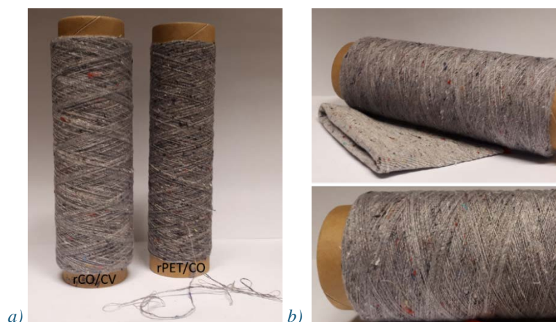
Figure 35 a) Yarns from 50 % r-CO (6) / 50 % CV (virgin) and 50 % r-PET / 50 % CO (virgin) and b) yarn and knitted sample from 30 % r-CO (5) / 70 % CV (virgin)
