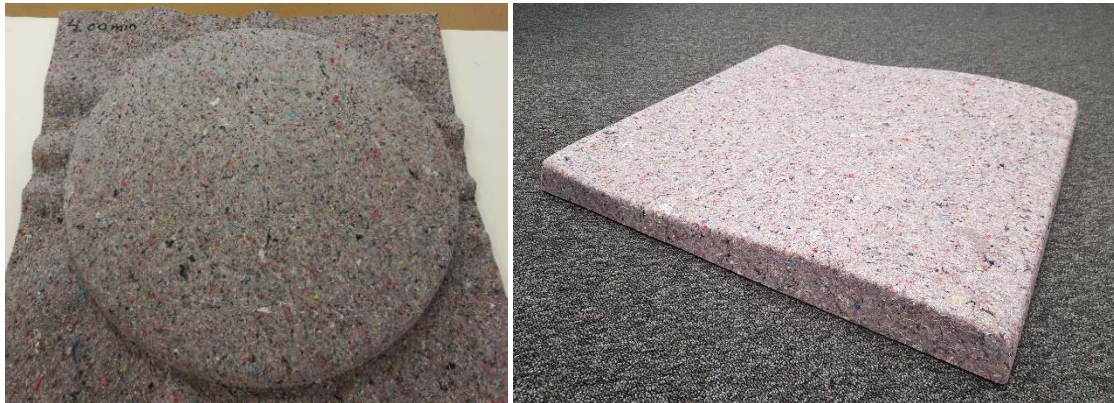
Figure 45 Acoustic panel prototypes produced from Laroche demo nonwovens
