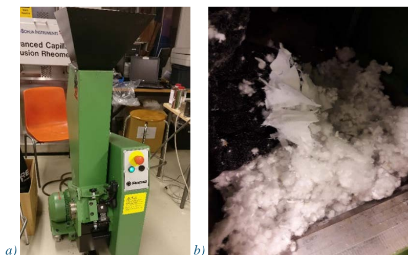
Figure 51 a) A crusher used in the trial was not effective enough to produce homogenous material. B) Large fabric pieces from the outer layers of pillows and duvets exist among polyester fibres after crushing
