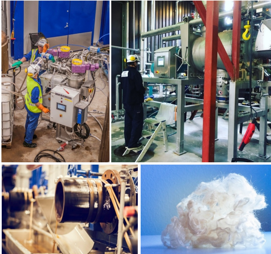
Figure 47 Generating viscose grade staple fibres from textile waste (Infinited Fibre Company)
