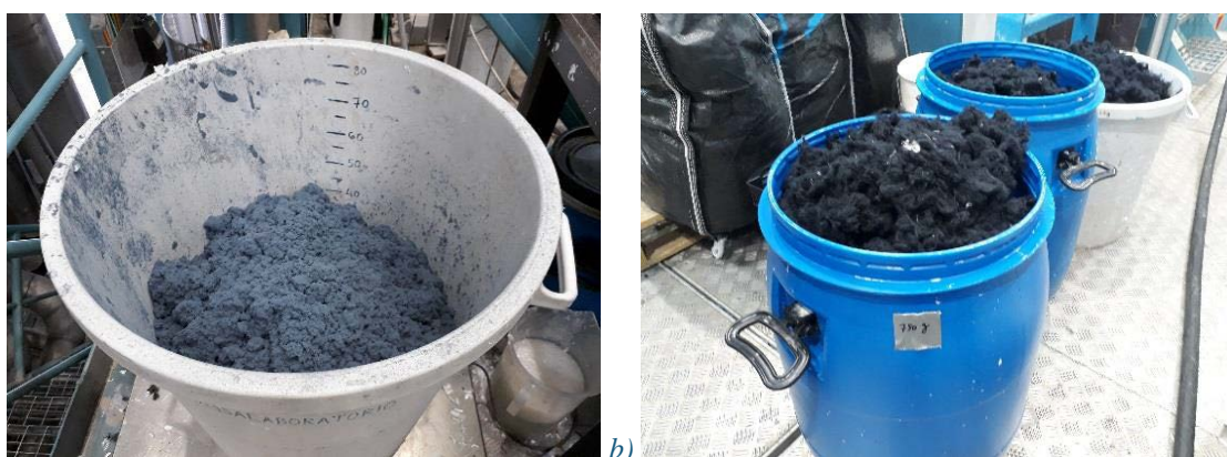
Figure 27 a) Cotton dust obtained as a waste fraction from mechanical recycling, and b) mechanical recycled cotton fibres
