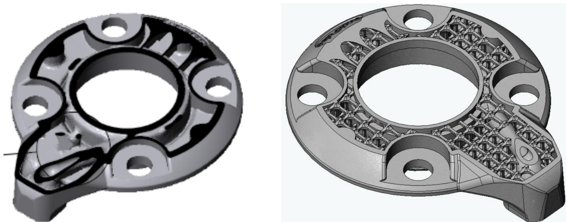
Figure 22. Enmac Oy pikehead component redesign examples utilizing topology optimization and lattice infill (Ahtiluoto, 2018).
