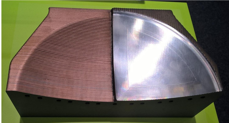
Figure 4. Big mold half (diameter about 500 mm). Two AM techniques have been used in the production of the piece. An inexpensive frame is built with a layer lamination. In this case, the laser-cut sheets with the cooling channels are joined together, and the final mold material is added to the coarse form by a DED (laser + powder). (Trumpf).
