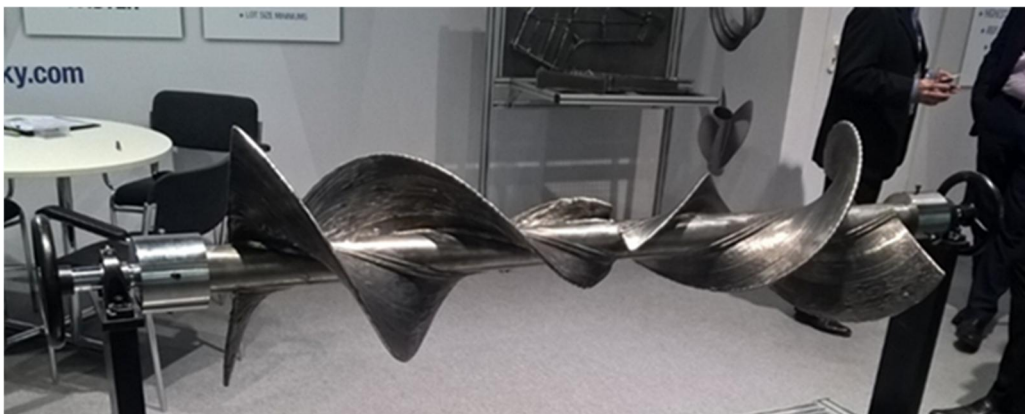
Figure 6. Features added by electron beam (Skiaky). The method can apply material up to 9 kg/h.
