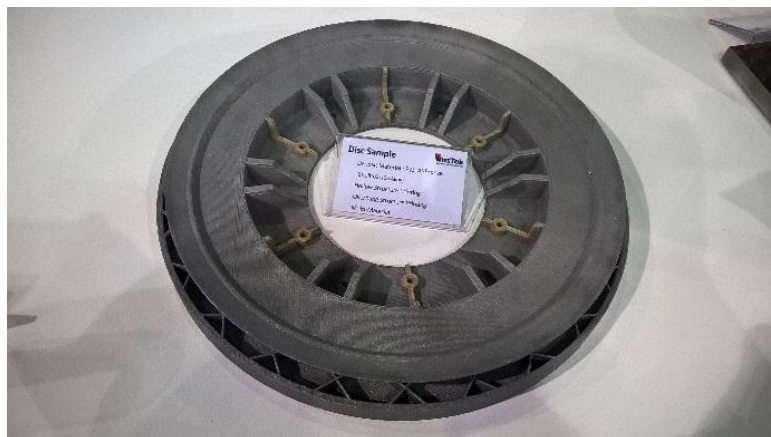
Figure 3. Multi-material disc, base material P21 and small details of aluminum bronze (Insstek).
