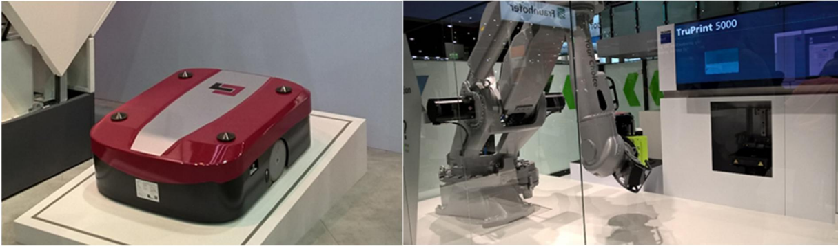
Figure 17. AGV concept from EOS (left) and Robotic handling of powder containers and building chambers by Trumpf (right).
