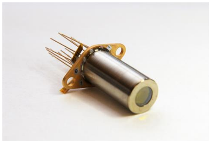
Figure 10. Assembled 2.65 \mu\text{m} source with an IR lens.
