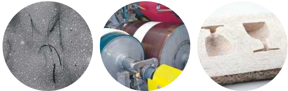
Figure. Fibre foam, foam formed board and an example of a porous foam product.
