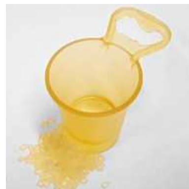
Figure 2. Demonstrated application by injection moulding based on VTT's thermoplastic cellulose.
