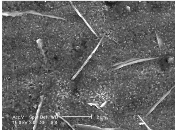
Fig. 2. A SEM of the surface of an oxidised TiAlN/VN coating sample 1, heat treated in air at 550 °C for 1 h.
