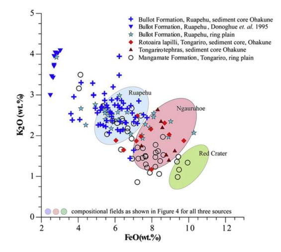
**Fig. 11.** Biplot of  $K_2O$  and FeO (total Fe expressed as FeO) derived by electron microprobe analyses of glass from tephras erupted from Ruapehu and Tongariro volcanoes younger than c. 12,000 cal. years, showing separation according to three sources (from Moebis et al., 2011, p. 359).
