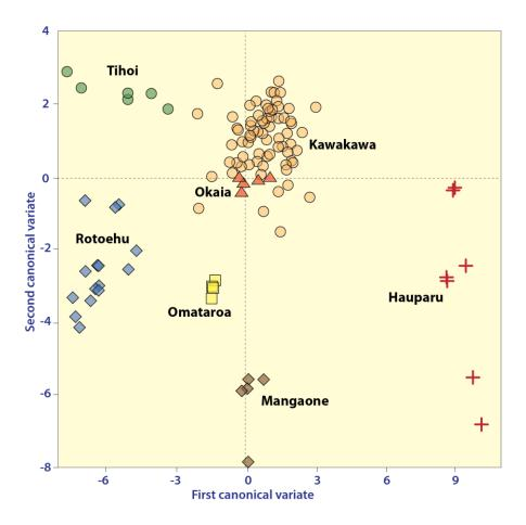
**Fig. 12.** Example of use of DFA to compare degree of similarity of seven late Quaternary rhyolitic tephras in central North Island, New Zealand. Glass compositions of each tephra were combined using DFA into the first two canonical variates. The Mahalanobis distance between groups  $(D_m^2)$  is a direct measure of their multivariate similarity/dissimilarity based on all seven major oxides analysed, not just two or three (from Lowe, 2011, after Cronin et al., 1997).
