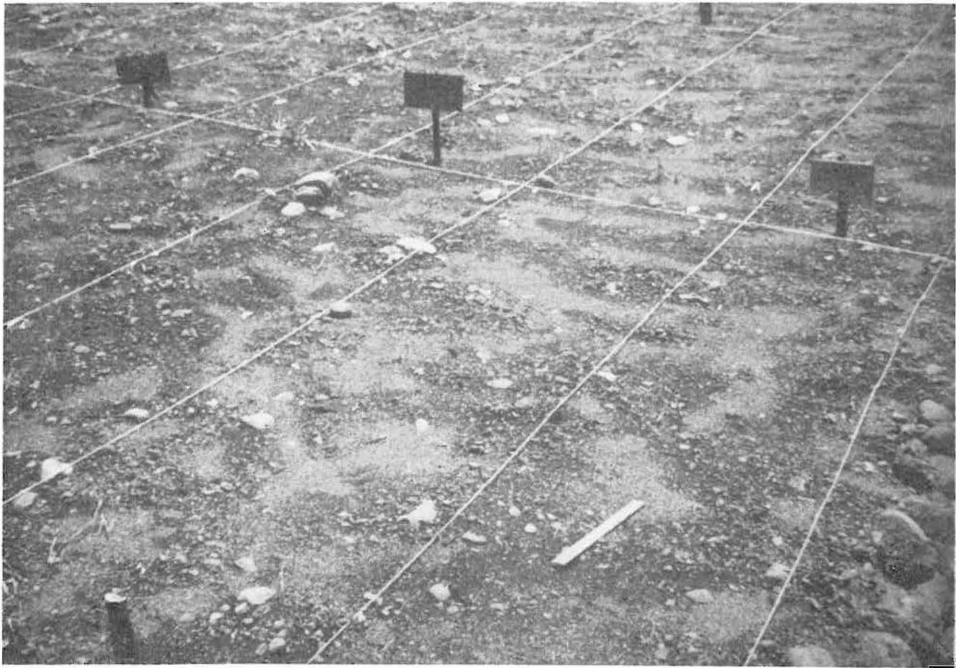
Figure 2 A typical soil crust showing surface 'dispersion mosaics'.
