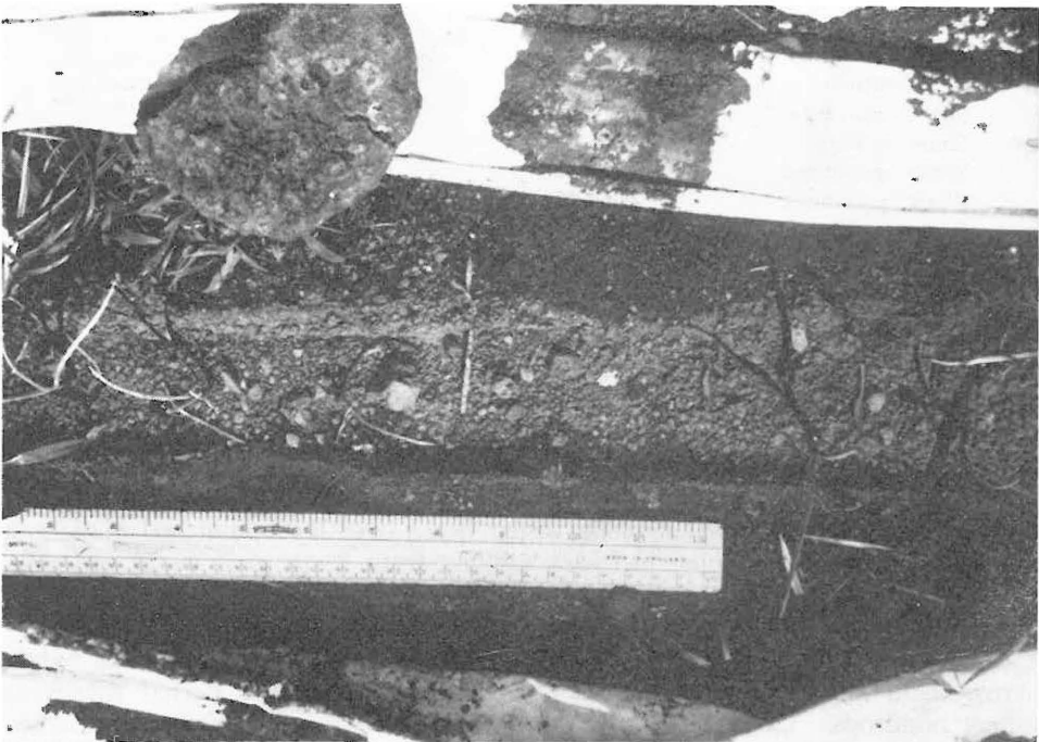
Figure 3 The lowering of the soil surface caused by soil crusting, in the exposed 3in wide area between two polythene sheets.
