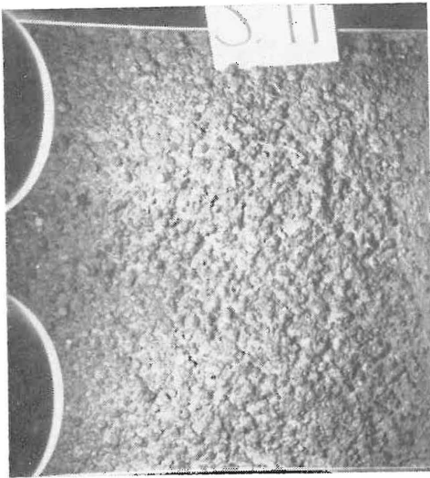
Figure 6A. Sample from A1 horizon of an iron-podzol after subjection to three periods of simulated rainfall, showing destruction of surface aggregation and puddling.
