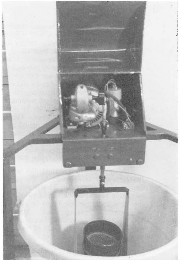
Figure 2. Detail of the wet-sieve aggregate analyzer, showing the electric motor, gearbox, crankshaft and bayonet junction.
