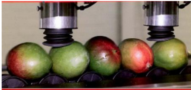
Figure 2-11. Mango fruit being measured for acoustic firmness using AWETA's online high-speed acoustic firmness sensor (AFS, AWETA, Nootdorp, Netherlands).
