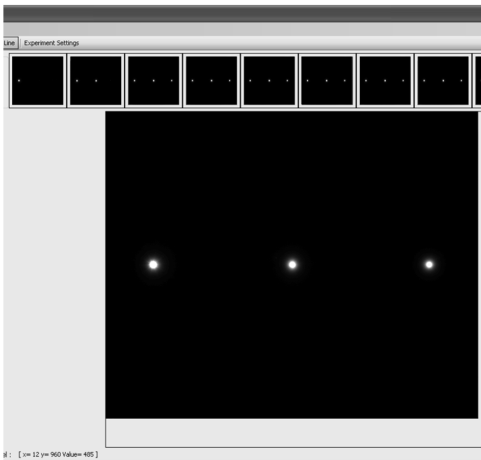
Figure 11-5. Software displaying thumbnails of images collected at the top and an example image in the main display. Note the three bright spots corresponding with the three lasers illuminating three different apples.
