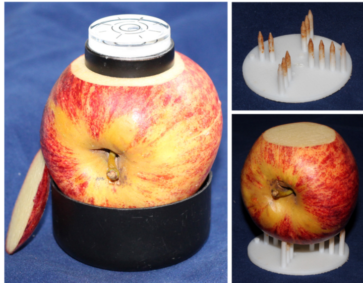
Figure 9-5. In the first position a black plastic cup was used to mount fruit. In the second position, when fruit had been sliced, a spiked mount was required.
