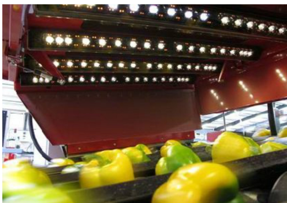
Figure 2-3. AWETA Powervision-3D lighting and camera system as seen from below (AWETA America, 2013).
