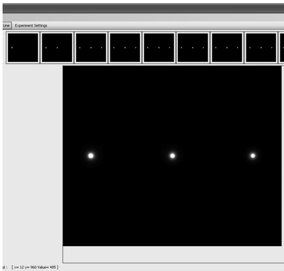
Figure 5-21. Software displaying thumbnails of images collected at the top and an example image in the main display. Note the three bright spots correspond with the three lasers illuminating three different apples.
