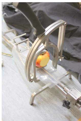
Figure 9-3. In-house designed 'guillotine' for making parallel slices on the fruit.
