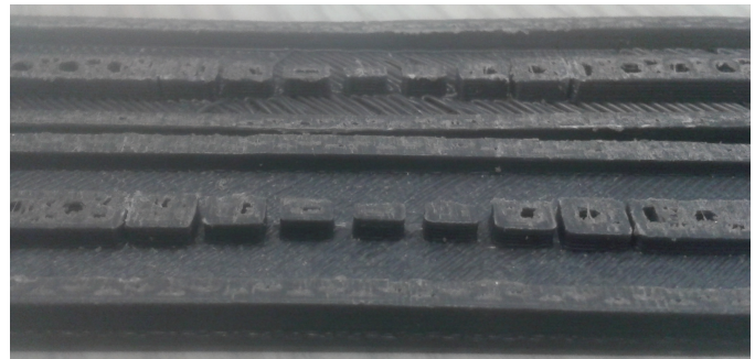
Fig. 5. MakeBot coupler cross section: At this angle inaccuracy in the internal geometry can be seen, the most extreme left and right wave guide portions are deformed and almost touching at points. The separation should be 0.276 mm or 276 microns.
