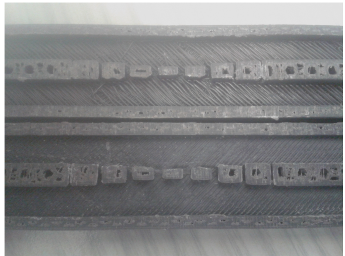
Fig. 4. Another MakeBot coupler, cross section: Cut with a band saw, poor surface finish can be seen on the roof of the coupler (upper half in the photo).
