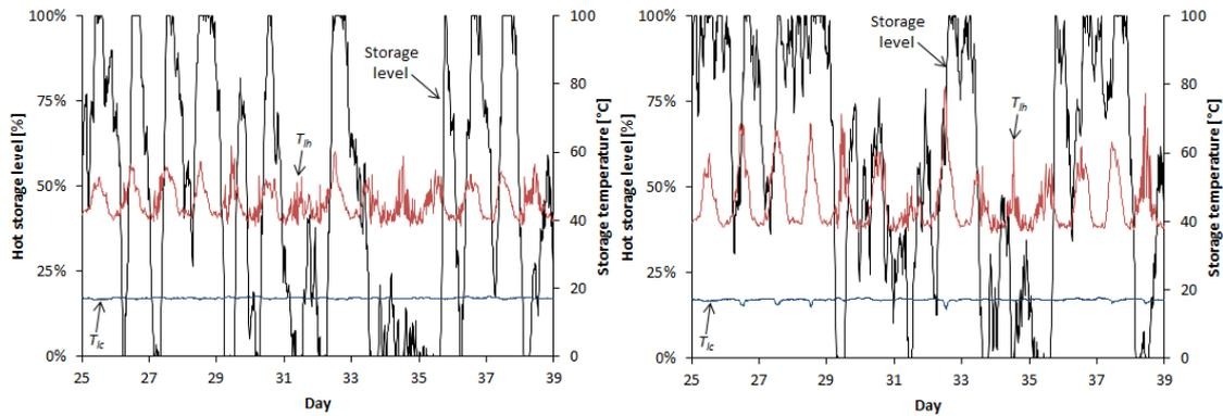
Figure 5: Hot storage tank levels and hot and cold storage tank temperatures for the Solar-HRL hybrid system with parallel solar (a, left) and return series solar (b, right), with 15,000 m<sup>2</sup> solar collector area and 500m<sup>3</sup> tank volume
