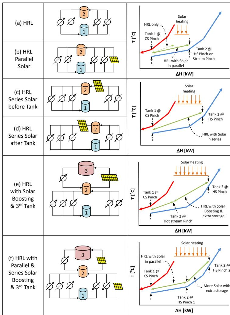
Figure 1: Solar-HRL hybrid system configurations and Composite Curves
