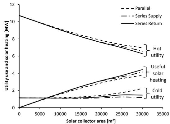
Figure 4: Solar-HRL hybrid system performance with constant hot and cold storage of 500 m<sup>3</sup>.
