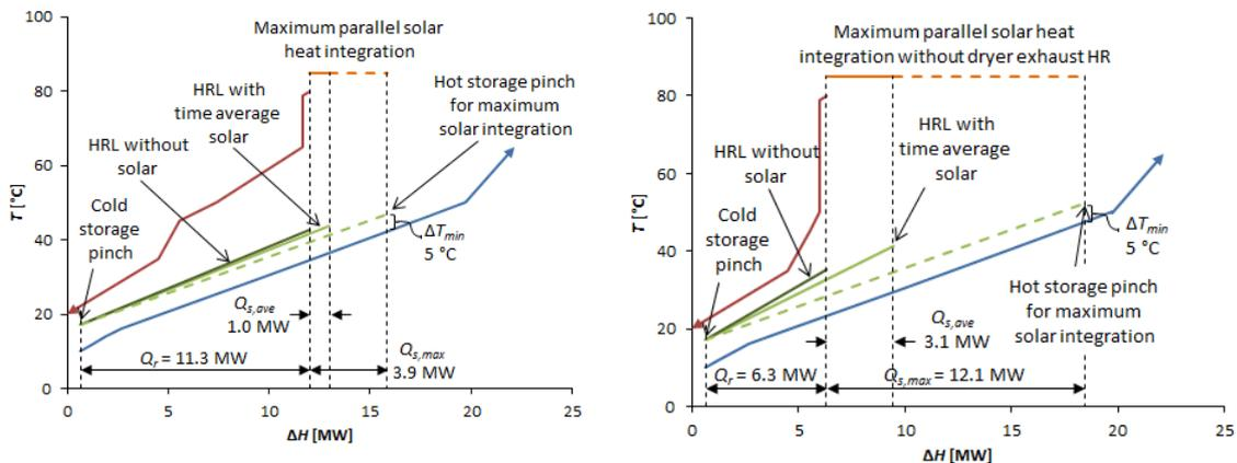
Figure 2: Composite Curves for Solar-HRL hybrid system with parallel solar collectors, with exhaust heat recovery (a, left) and without exhaust heat recovery (b, right)
