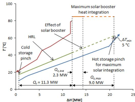
Figure 3: Composite curves for Solar-HRL hybrid system with series solar collectors.
